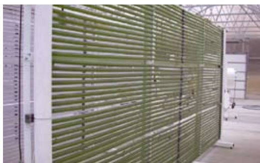
Figure 6 Tubular photobioreactor, image courtesy of Varicon Aqua Solutions Ltd UK.
