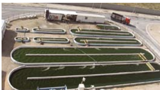
Figure 5 Example of an open raceway pond culture system (Seambiotic, Israel)
